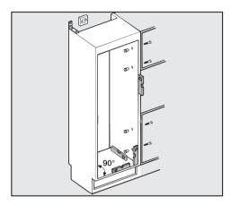
Use a spirit level to align the housing unit.
